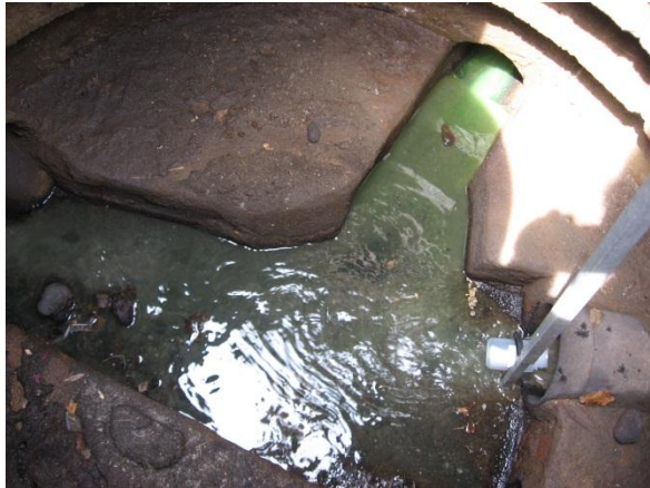
Photos of the manhole outside of the Calf Pasture Beach concession stand. The green substance is the result of a dye test which proved that the concession stand was connected to the storm drain system and not the sewer (Above). After the smoke test showed that all drains in the concession stand we're connected to the storm drain system, they we're plugged to prevent any further leaking before the lines were rerouted (Right).
